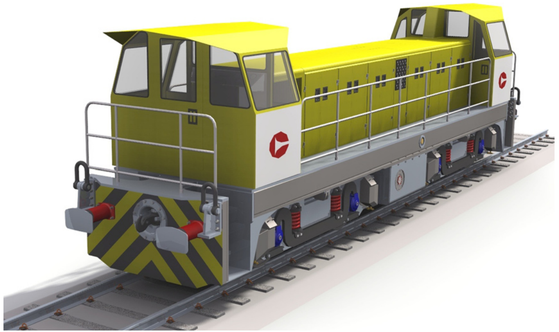
ABOVE: A Computer Aided Design drawing of one of the twin-cabbed modular bogie diesel locomotives. Corus
